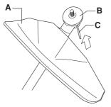
Screw on the trimmer head/plastic blades (H) in the opposite direction to the direction of rotation.
